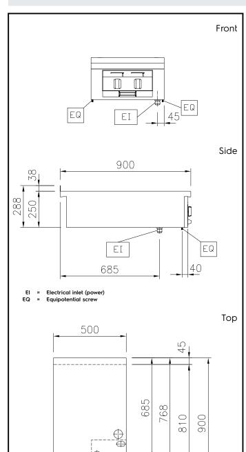
**Electric** Supply voltage: 400 V/3N ph/50/60 Hz Total Watts: 6 kW **Key Information: Working Temperature MIN:** 100 °C **Working Temperature MAX:** 450 °C 500 mm External dimensions, Width: External dimensions, Depth: 900 mm External dimensions, Height: 250 mm Net weight: 75 kg Configuration: One-Side Operated;Top Front Plates Power: 3 - 0 kW **Back Plates Power:** 3 - kW Solid top usable surface 360 mm (width): Solid top usable surface
